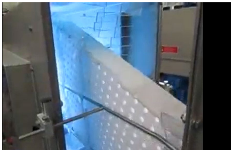
Example of Trays Surface UV-C Treatment with Light Progress devices.
