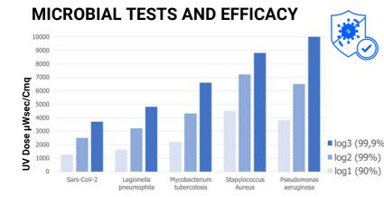
Up-to log3 microbial reduction on Airflow, Coils and HVAC surfaces, 24 hours a day.
