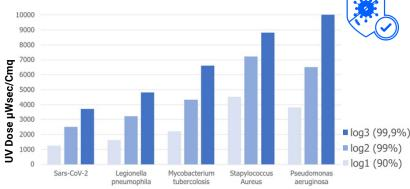
Up-to log3 microbial reduction on Airflow, Coils and HVAC surfaces, 24 hours a day.
